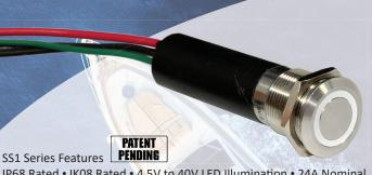
IP68 Rated • IK08 Rated • 4.5V to 40V LED Illumination • 24A Nominal Load Current • 6V to 26.4V DC Voltage • Rated to >1,000,000 On-Off Cycles • Short Circuit Protection with Latch • Overload Protection • Thermal Shutdown with Latch • In-rush Current Protected • Reverse **Battery Protection**
